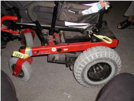
< Wheelchair with tether straps installed
