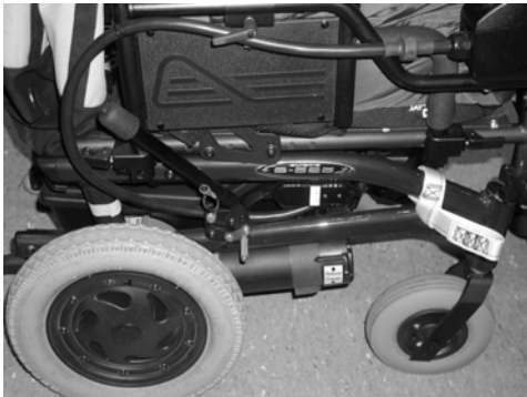
< Wheelchair with markings (rear) and tether straps (front)
